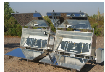
Type F3 (Arizona) - dual axis tracking (elevation and azimuth), and dual mirrors
