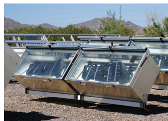
Type F2 (Arizona) - fixed elevation, tracking azimuth
