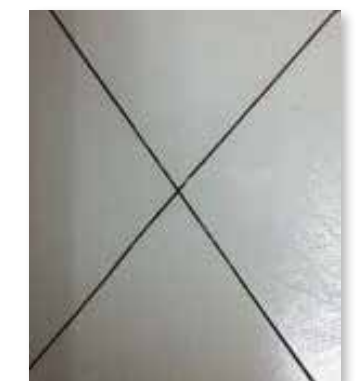
Paint applied to aluminum with pre-treatment B shows excellent adhesion performance
