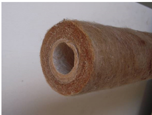
Microporous depth filter after one month of use at Q-Lab Arizona.
