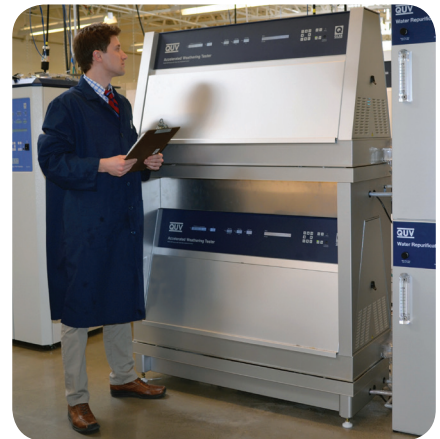
Stacking testers on the space saver frame allows easy access to both machines.
