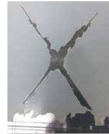
Aluminum panel made from alloy Y shows poor adhesion & significant delamination of paint from the surface
