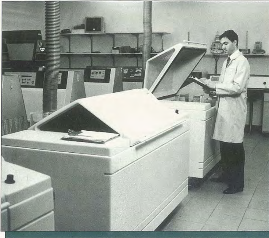
Cyclic corrosion test cabinets are used for new standards that require cyclic exposure to salt, fog, dry-off and humidity.
