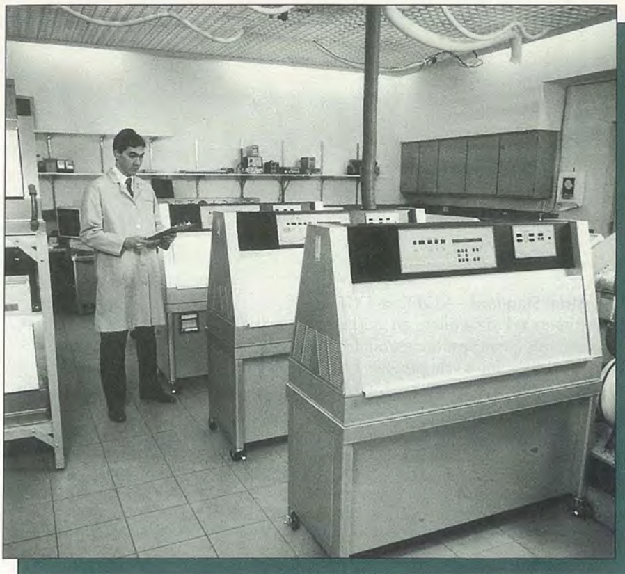
ASTM D 5894 calls for UV exposure cabinets in combination with cyclic salt fog cabinets.
