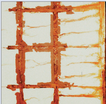
Left Front Fender; 192 hours, salt spray
