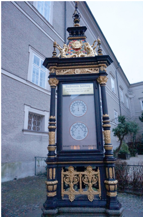
This late 19th century weather station in Salzburg, Austria was declared an historical landmark in 2007. Pictured is the side displaying the relative humidity. Hygrometers of this era commonly used human hair under tension, which changes length depending on the moisture content of the air.
