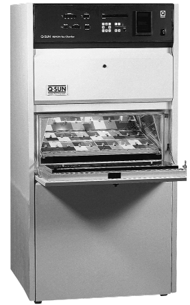
The Q-Sun's full-spectrum xenon arc lamps emit UV, visible light and infrared.
