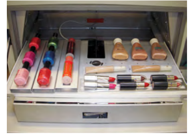
Bottles and other oddly-shaped samples can be easily tested in a Q-SUN chamber due to its flat specimen tray and variety of mounting options.
