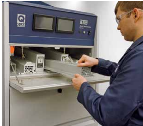
Q-SUN chamber lamp replacement is almost effortless: just open the hinged door, disconnect and slide out the lamp.
