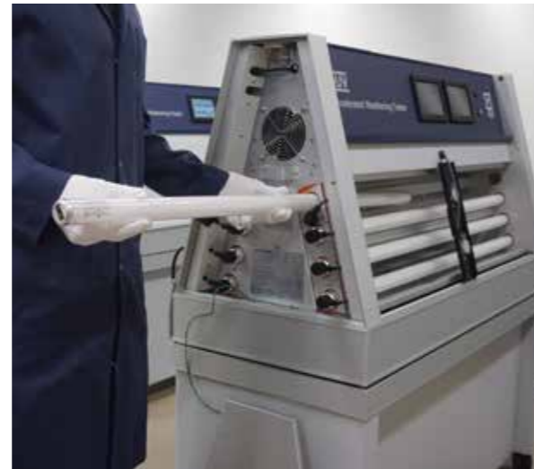
Irradiance-controlled QUV models do not require lamp rotation. However, when the time comes to replace a lamp, double sided access makes the job easy to perform.
