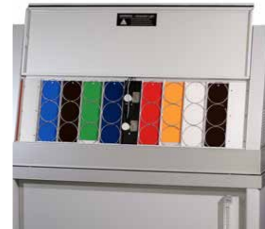
A QUV tester can accommodate 48 specimens.
