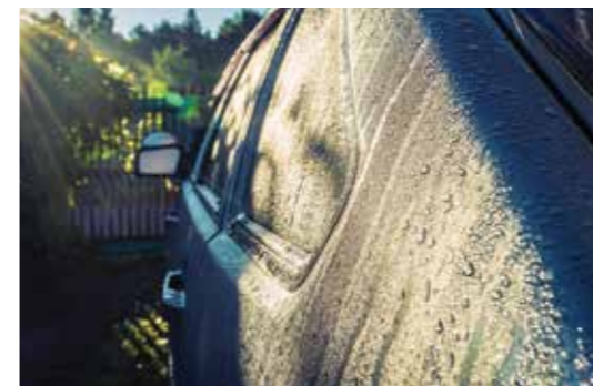
Products exposed outdoors often remain wet 8-12 hours each day. Dew, not rain, is responsible for most of the damage caused by outdoor wetness.
